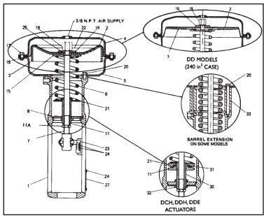
Parts For Models RA, RB, RC and RD — Reverse-Acting
