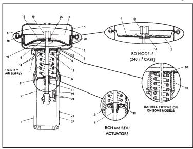
Type II Override/Limit Stop Assembly For Reverse-Acting Actuator
