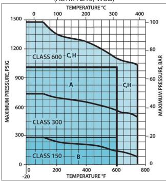
Figure 3. Trim Chart For Chrome-Moly Body (ASTM A217, C5)
